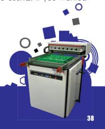
to produce 500 parts in one go then usually this kind of part would be produced two up on one of our larger machines. The benefits of increasing the number of tools used to form the parts is that the job is completed in a shorter time and so you have reduced labour and machine costs and in addition when multiples of tools are used, it usually means that less material is wasted.
